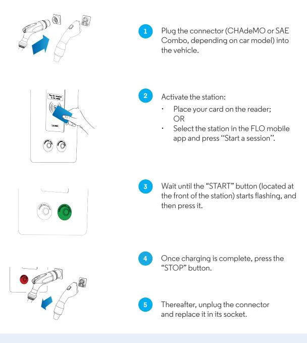
**IMPORTANT :** Once charging is complete, make sure to wind the cable and store the connector in its socket.
