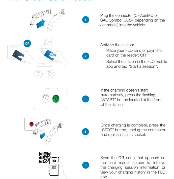
**IMPORTANT:** Once charging is complete, make sure to wind the cable and store the connector in its socket.
