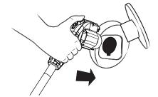
Plug the connector into your vehicle. Charging will start immediately.
