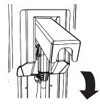
Once charging is complete, unplug the connector, replace it in its socket and close the door.
